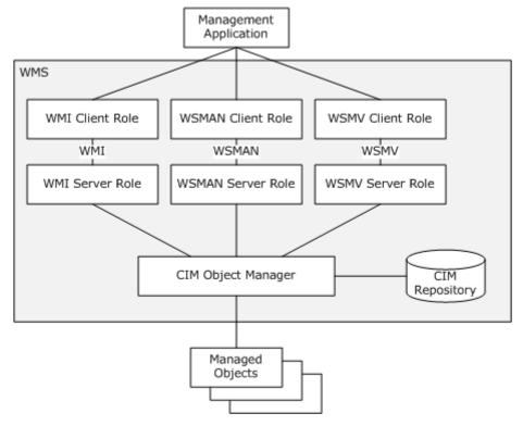
Figure 16: WMS internal architecture
