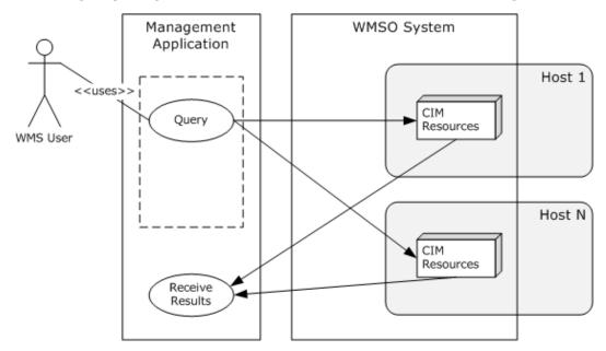
Figure 8: Querying properties of a CIM instance
