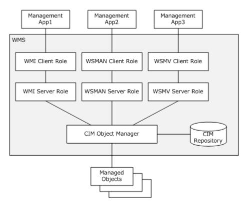
Figure 13: WMS System as CIM data interface
