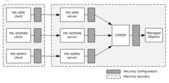
Figure 22: Security configuration settings
