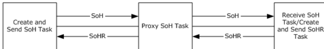
Figure 69: Message flow between the NAP client and the NAP health policy server
