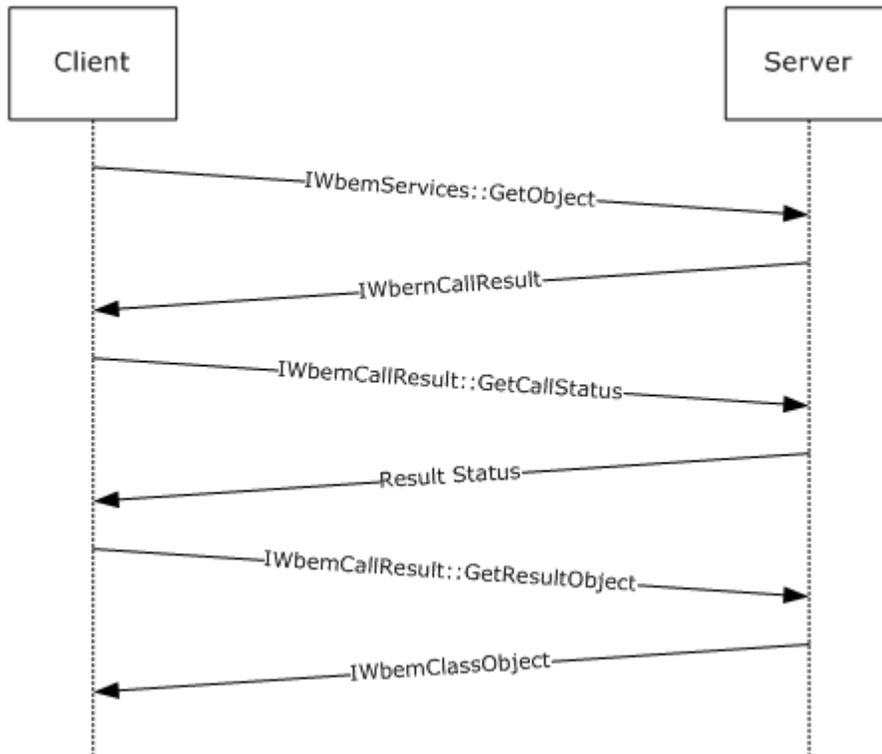
Figure 17: Semisynchronous delivery of a single result
