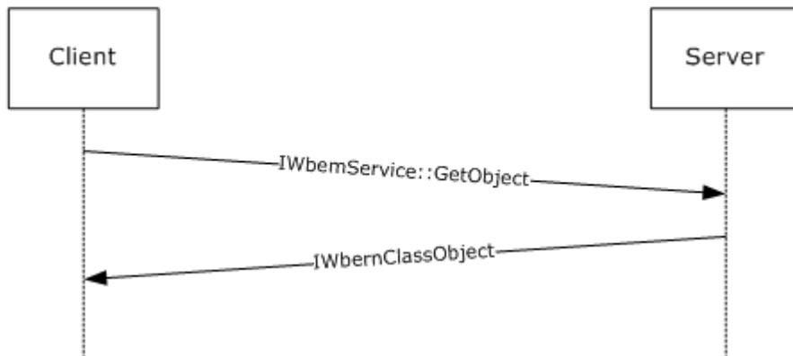
**Figure 12: Synchronous delivery of a single result**
