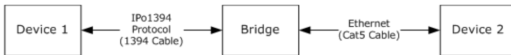
Figure 1: IPo1394 in environment where the IPo1394 network is bridged to an Ethernet network
