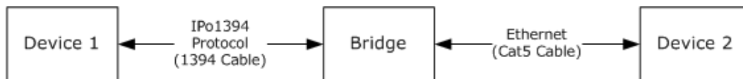
Figure 1: IPo1394 in environment where the IPo1394 network is bridged to an Ethernet network
