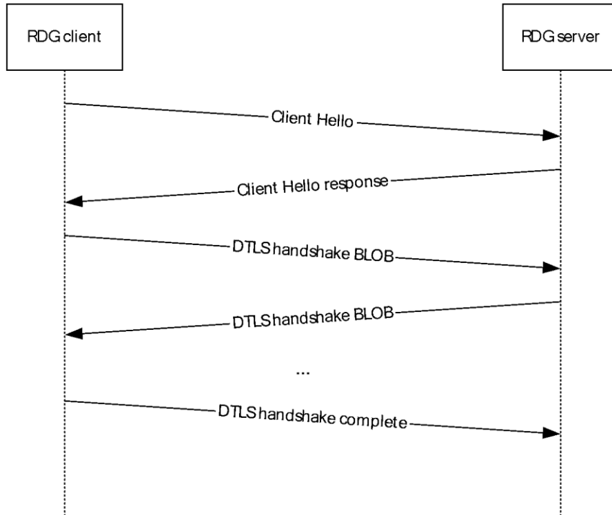
Figure 9: Message sequence between RDG client and RDG server during DTLS handshake phase
