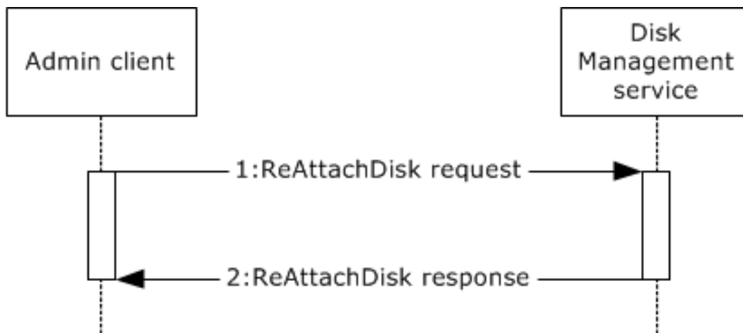
Figure 8: Example of making an offline disk into an online disk
