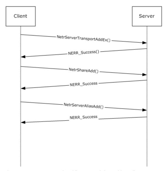
Figure 3: Message sequence for adding a scoped share with an alias to a server
