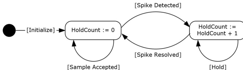
**Figure 5: Client spike evaluation and processing**
