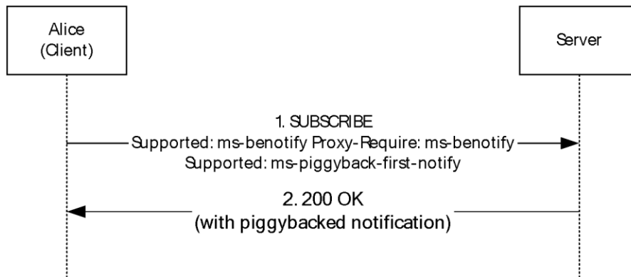
Figure 3: Batched SUBSCRIBE request and piggybacked NOTIFY example
