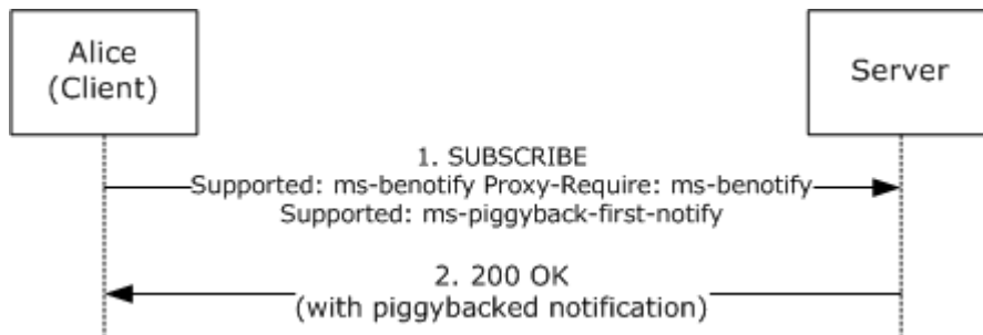
Figure 3: Batched SUBSCRIBE request and piggybacked NOTIFY example
