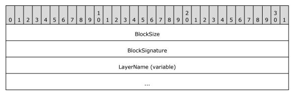
**BlockSize (4 bytes):** A 32-bit, unsigned integer that specifies the size of the ShimDataBlock structure. This value MUST be greater than or equal to 0x00000088.
