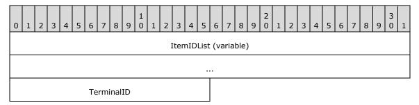
ItemIDList (variable): An array of zero or more ItemID structures (section 2.2.2).
