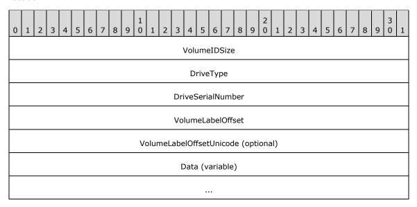
**VolumeIDSize (4 bytes):** A 32-bit, unsigned integer that specifies the size, in bytes, of this structure. This value MUST be greater than 0x00000010. All offsets specified in this structure
