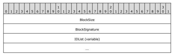
**BlockSize (4 bytes):** A 32-bit, unsigned integer that specifies the size of the VistaAndAboveIDListDataBlock structure. This value MUST be greater than or equal to 0x0000000A.
