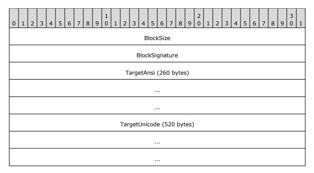
**BlockSize (4 bytes):** A 32-bit, unsigned integer that specifies the size of the IconEnvironmentDataBlock structure. This value MUST be 0x00000314.
