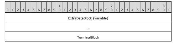
**ExtraDataBlock (variable):** An optional array of bytes that contains zero or more property data blocks listed in the **EXTRA\_DATA\_BLOCK** syntax rule.
