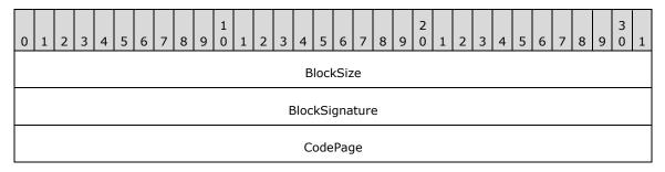
**BlockSize (4 bytes):** A 32-bit, unsigned integer that specifies the size of the ConsoleFEDataBlock structure. This value MUST be 0x0000000C.
