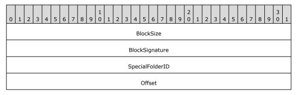
**BlockSize (4 bytes):** A 32-bit, unsigned integer that specifies the size of the SpecialFolderDataBlock structure. This value MUST be 0x00000010.
