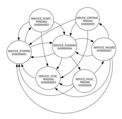
Figure 1: State Diagram in which life cycle and execution properties are governed by the rules defined in  $\mathsf{SCM}$
