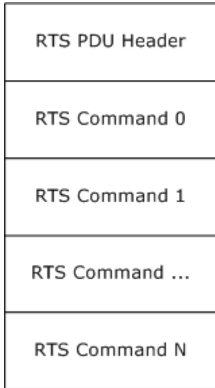
Figure 12: RTS PDU structure
