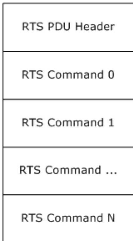
Figure 12: RTS PDU structure
