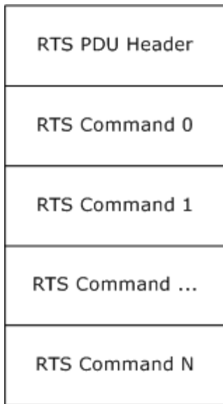
Figure 12: RTS PDU structure
