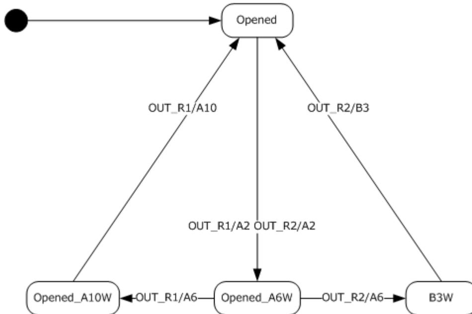
**Figure 26: Client virtual OUT channel state machine**
