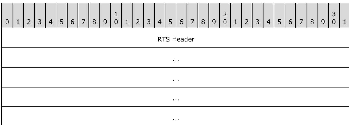
**RTS Header (20 bytes):** See section [2.2.3.6.1](#). The **Flags** field of the RTS Header MUST be the value RTS\_FLAG\_PING. The **NumberOfCommands** field of the RTS Header MUST be the value 0.
