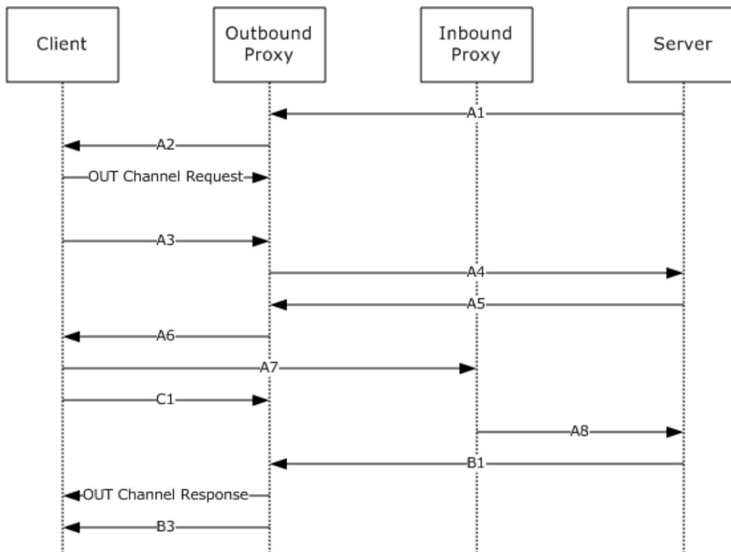
**Figure 21: OUT channel recycling 2 protocol sequence**
