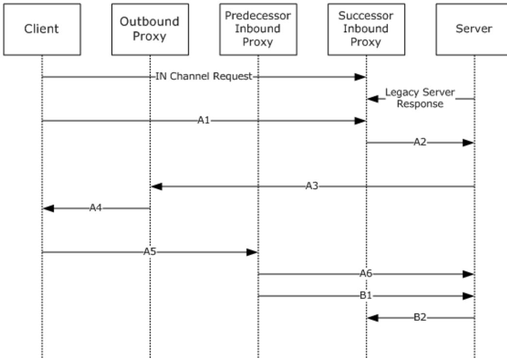
**Figure 18: IN channel recycling 1 protocol sequence**
