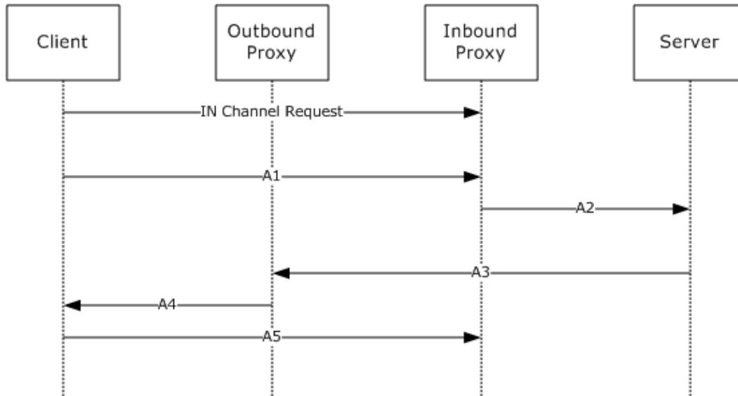
**Figure 19: IN channel recycling 2 protocol sequence**
