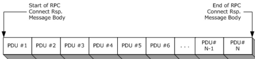
**Figure 9: Outbound RPC connect response PDU stream**
