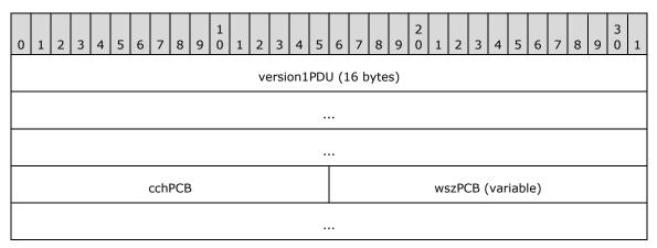
**version1PDU (16 bytes):** The RDP\_PRECONNECTION\_PDU\_V1 header, as specified in section 2.2.1.1.
