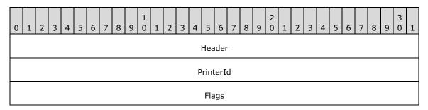
**Header (4 bytes):** The common message header (as specified in [MS-RDPEFS] section 2.2.1.1). The **Component** field MUST be set to RDPDR\_CTYP\_PRN and the **PacketId** field MUST be set to PAKID PRN USING XPS.
