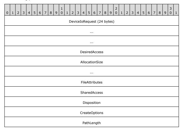
**DeviceIoRequest (24 bytes):** A DR\_DEVICE\_IOREQUEST header (as specified in [MS-RDPEFS] section 2.2.1.4).
