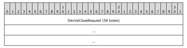
**DeviceCloseRequest (56 bytes):** A DR\_CLOSE\_REQ message (as specified in [MS-RDPEFS] section 2.2.1.4.2). This request closes a printer opened by DR\_PRN\_CREATE\_REQ (section 2.2.2.7).
