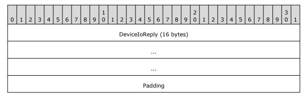
**DeviceIoReply (16 bytes):** A DR\_DEVICE\_IOCOMPLETION header (as specified in [MS-RDPEFS] section 2.2.1.5). The **CompletionId** field of this header MUST match the **CompletionId** of a Device I/O Request message that had the **MajorFunction** field set to IRP\_MJ\_CLOSE.
