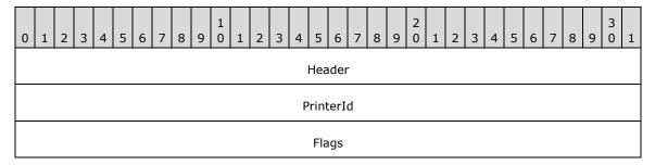
**Header (4 bytes):** The common message header (as specified in [MS-RDPEFS] section 2.2.1.1). The **Component** field MUST be set to RDPDR\_CTYP\_PRN and the **PacketId** field MUST be set to PAKID\_ PRN\_USING\_XPS.
