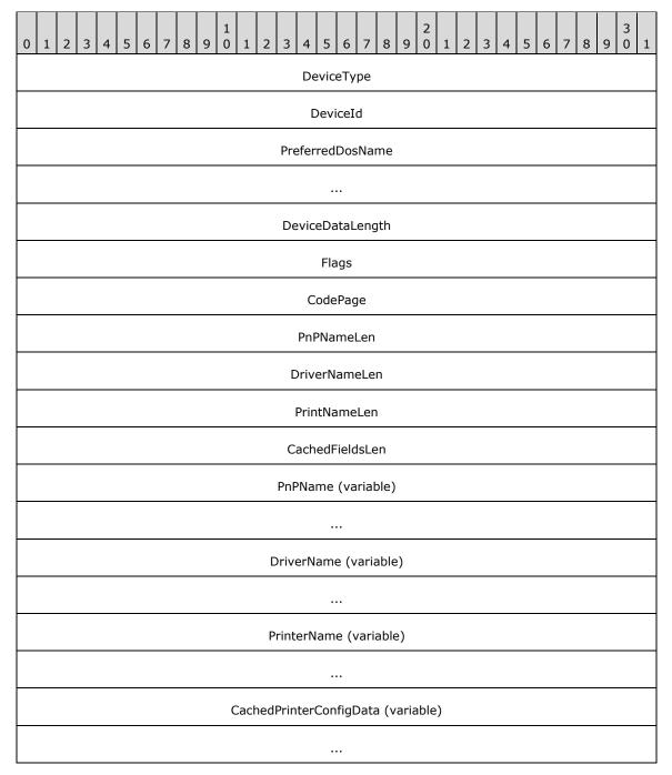
**DeviceType (4 bytes):** This field is defined in [MS-RDPEFS] section 2.2.1.3. This field MUST be set to RDPDR DTYP PRINT.
