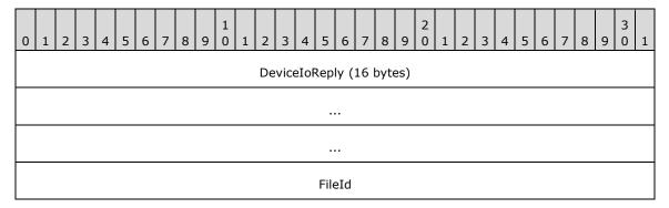
**DeviceIoReply (16 bytes):** A DR\_DEVICE\_IOCOMPLETION header (as specified in [MS-RDPEFS] section 2.2.1.5). The **CompletionId** field of this header MUST match the **CompletionId** of a Device I/O Request message that had the **MajorFunction** field set to IRP\_MJ\_CREATE.
