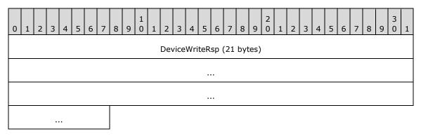
**DeviceWriteRsp (21 bytes):** A DR\_WRITE\_RSP request (as specified in [MS-RDPEFS] section 2.2.1.5.4). The **Length** field of this response is equal to the **Length** field of the Write Request (as specified in [MS-RDPEFS] section 2.2.3.3.4).
