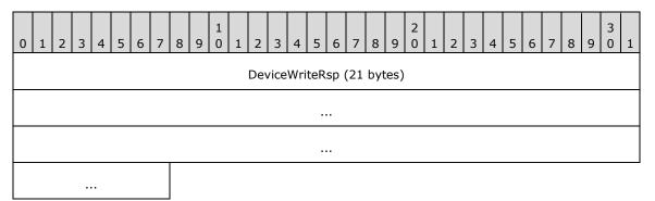
**DeviceWriteRsp (21 bytes):** A DR\_WRITE\_RSP request (as specified in [MS-RDPEFS] section 2.2.1.5.4). The **Length** field of this response is equal to the **Length** field of the Write Request (as specified in [MS-RDPEFS] section 2.2.3.3.4).
