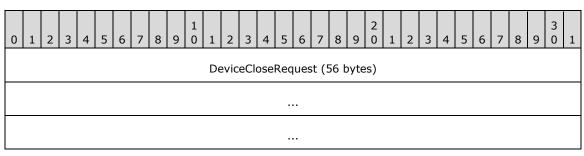
**DeviceCloseRequest (56 bytes):** A DR\_CLOSE\_REQ message (as specified in [MS-RDPEFS] section 2.2.1.4.2). This request closes a printer opened by DR\_PRN\_CREATE\_REQ (section 2.2.2.7).
