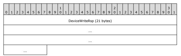
**DeviceWriteRsp (21 bytes):** A DR\_WRITE\_RSP request (as specified in <u>[MS-RDPEFS]</u> section 2.2.1.5.4). The **Length** field of this response is equal to the **Length** field of the Write Request (as specified in [MS-RDPEFS] section 2.2.3.3.4).
