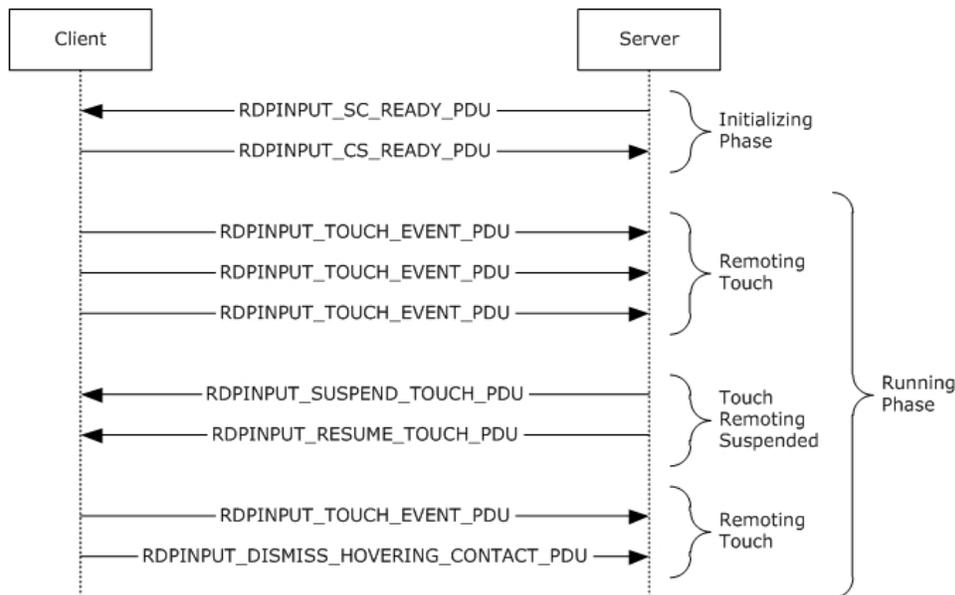
**Figure 1: Messages exchanged by the Input Protocol endpoints**
