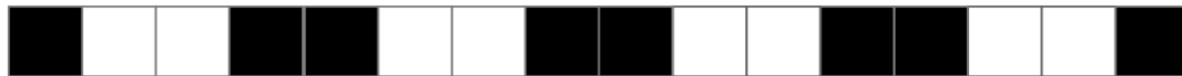
Figure 10: Sixteen glyph pixels stored in a linear stream with no implied dimensions
