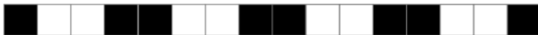
Figure 10: Sixteen glyph pixels stored in a linear stream with no implied dimensions
