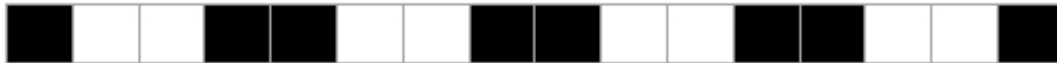
Figure 10: Sixteen glyph pixels stored in a linear stream with no implied dimensions
