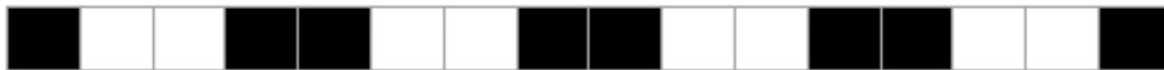
Figure 8: Sixteen glyph pixels stored in a linear stream with no implied dimensions
