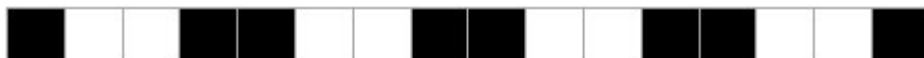
Figure 6: Sixteen glyph pixels stored in a linear stream with no implied dimensions
