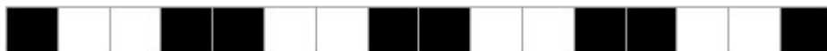
Figure 7: Sixteen glyph pixels stored in a linear stream with no implied dimensions
