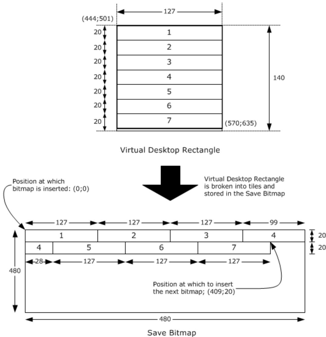
**Figure 20: Illustration of Save Bitmap Primary Drawing Order**
