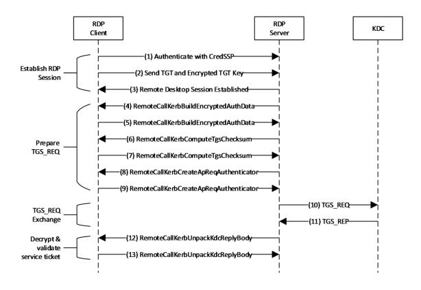
Figure 1: Sequence diagram for requesting a service ticket over RDP using RDPEAR
