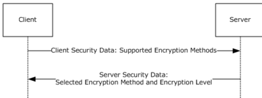
Figure 8: Determining the cryptographic configuration for a session
