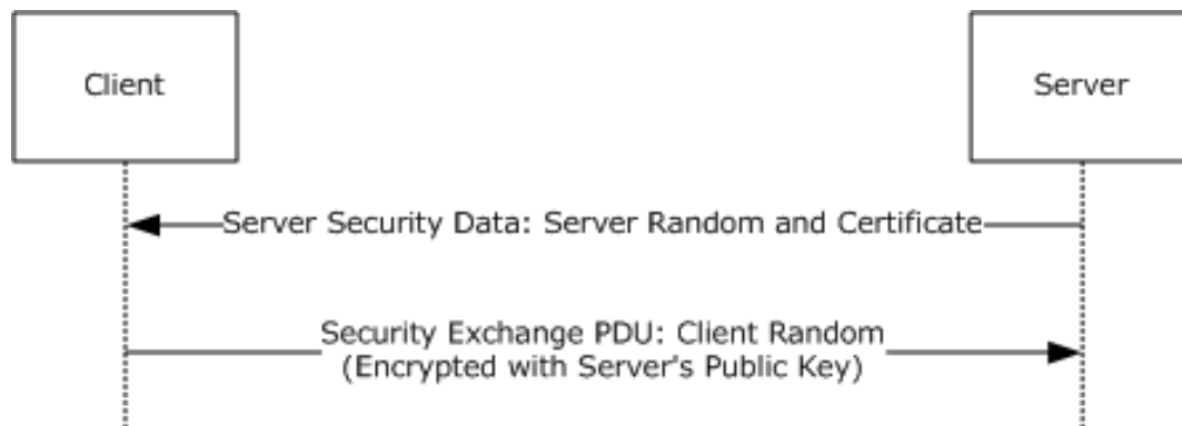
Figure 9: Client and server random value exchange
