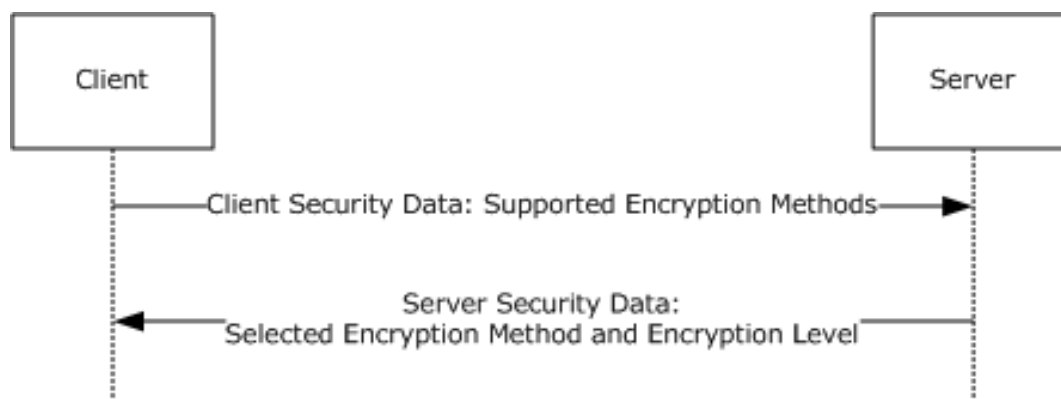
Figure 8: Determining the cryptographic configuration for a session
