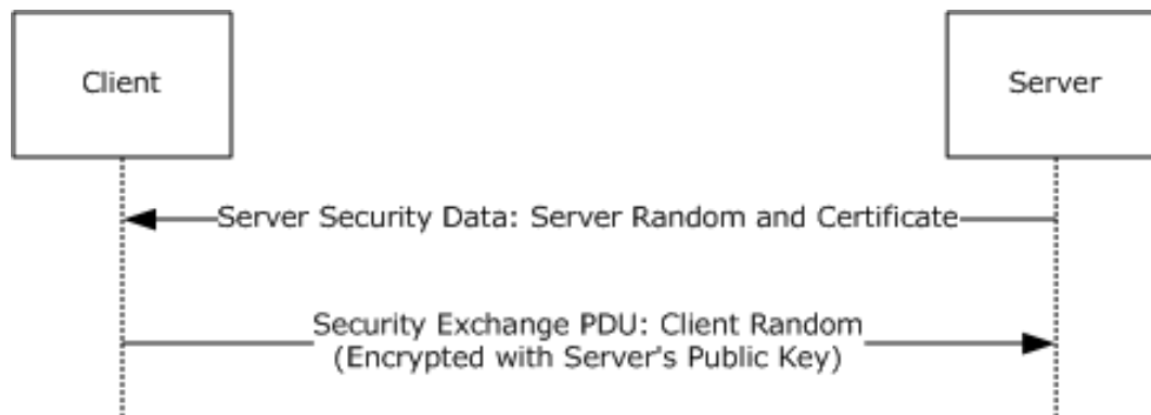
Figure 8: Client and server random value exchange
