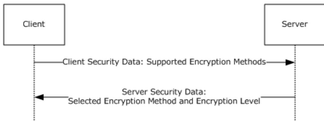
Figure 7: Determining the cryptographic configuration for a session
