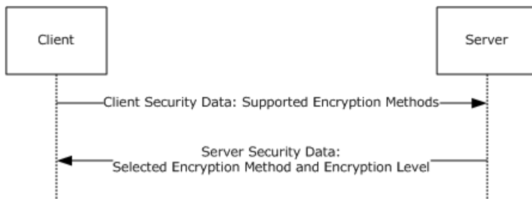
Figure 7: Determining the cryptographic configuration for a session
