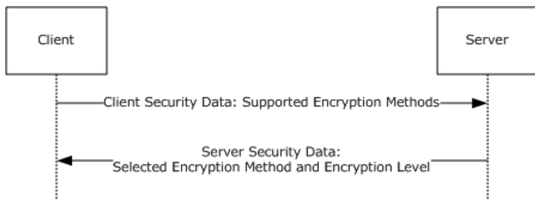
Figure 7: Determining the cryptographic configuration for a session
