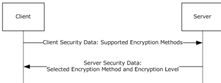
Figure 7: Determining the cryptographic configuration for a session
