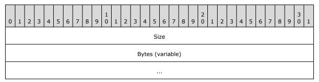
Size (4 bytes): The size in bytes of the Bytes field, not including padding (if any).
