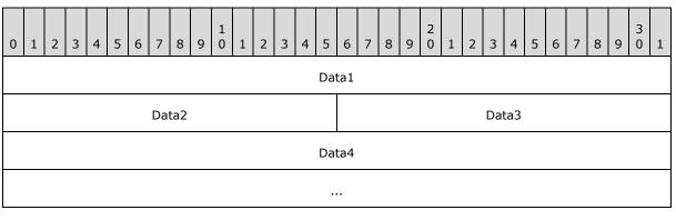
Data1 (4 bytes): The value of the Data1 field specified in [MS-DTYP] section 2.3.4.
