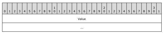
Value (8 bytes): The value of the DATE is an 8-byte IEEE floating-point number, as specified in [MS-OAUT] section 2.2.25.
