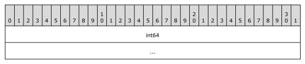
int64 (8 bytes): The value of the int64 field specified in [MS-OAUT] section 2.2.24.
