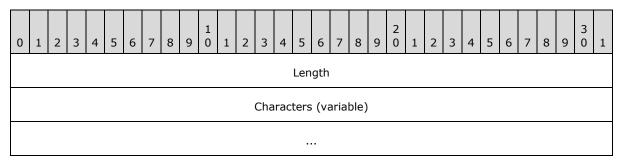
**Length (4 bytes):** The length in 16-bit Unicode characters of the **Characters** field, including the null terminator, but not including padding (if any).
