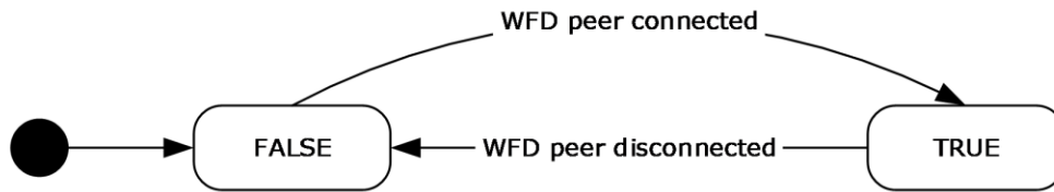
Figure 6: OOB Connector WFDPeerConnected transitions
