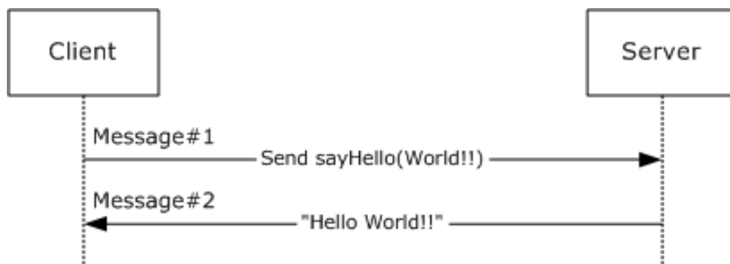
Figure 17: Sequence diagram for Hello World!!
