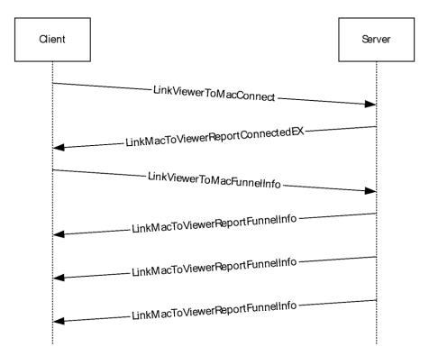
Figure 5: Packet-pair commands for TCP connections
