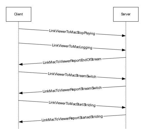
Figure 7: Sequencing during playback--fast forward and rewind buttons
