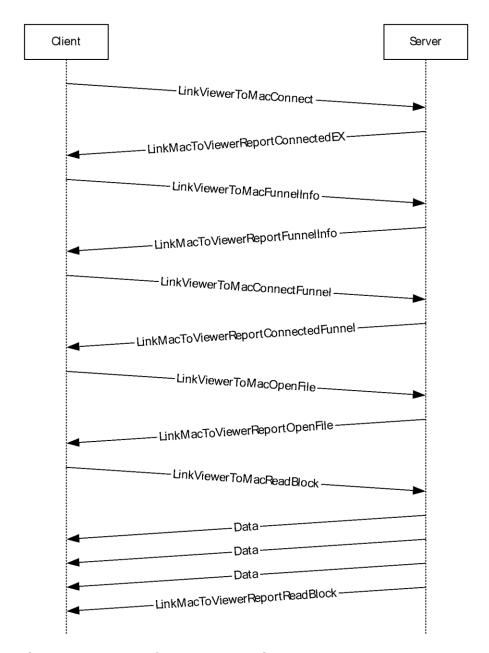
Figure 4: Sequence for UDP connections
