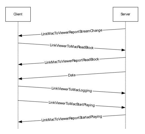
Figure 8: Sequencing during playback--server changes streams
