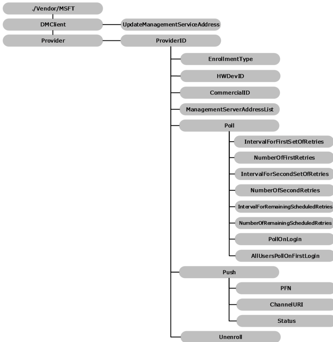
Figure 5: The DMClient configuration service provider in tree format
