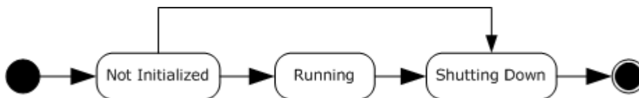
Figure 5: State machine diagram for the server
