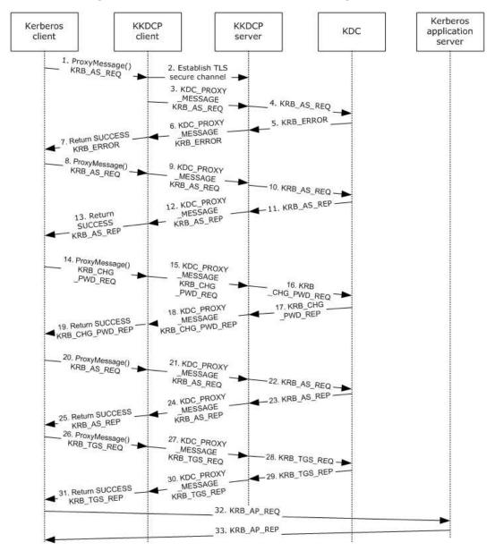
Figure 3: Obtaining a service ticket with password change
