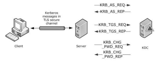
Figure 1: Messages between client, server, and KDC
