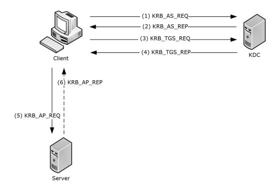
Figure 1: Kerberos V5 Exchanges
