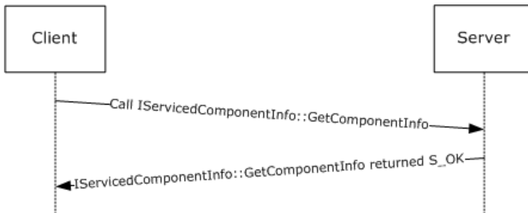
Figure 4: Call sequence for determining server object identity
